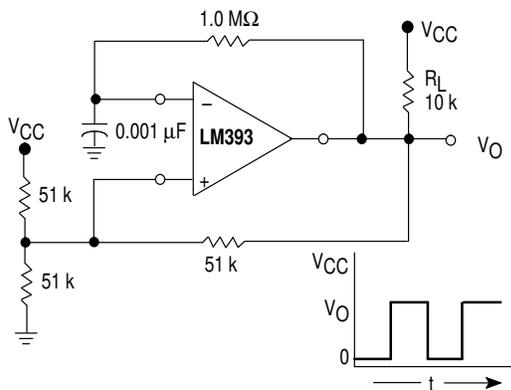
**Figure 10. Time Delay Generator**
