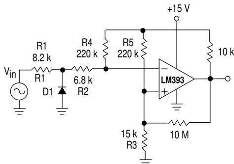
D1 prevents input from going negative by more than  $0.6\text{ V}$ .
