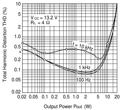
Figure 5 Total Harmonic Distortion vs. Output Power
