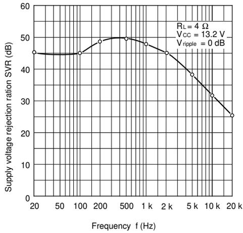
Figure 7 Supply Voltage Rejection Ratio vs. Frequency
