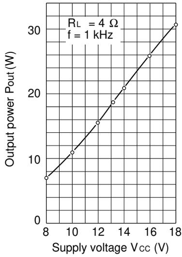
Figure 2 Output Power vs. Supply Voltage
