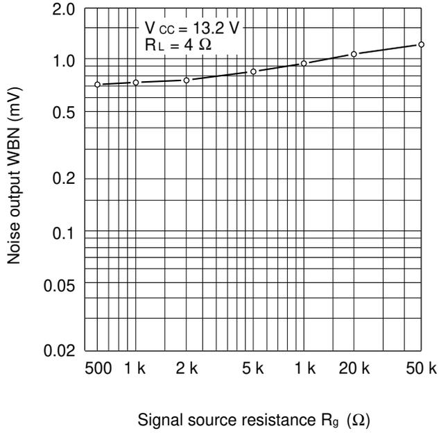
Figure 6 Noise Output vs. Signal Source Resistance
