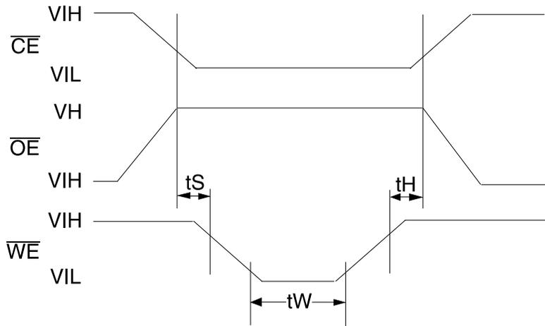
t<sub>S</sub> = t<sub>H</sub> = 1  $\mu$ sec (min.)
