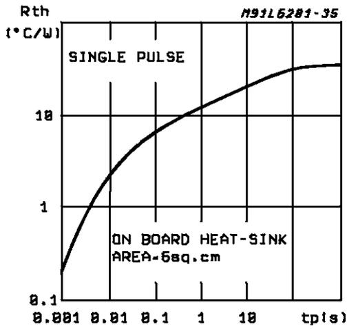
**Figure 25:** Typical  $R_{Th J-amb}$  of Multiwatt Package vs. Total Power Dissipation
