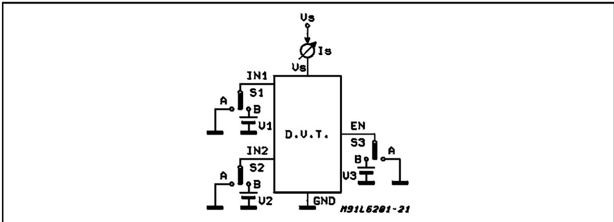
Figure 11: Leakage Current
