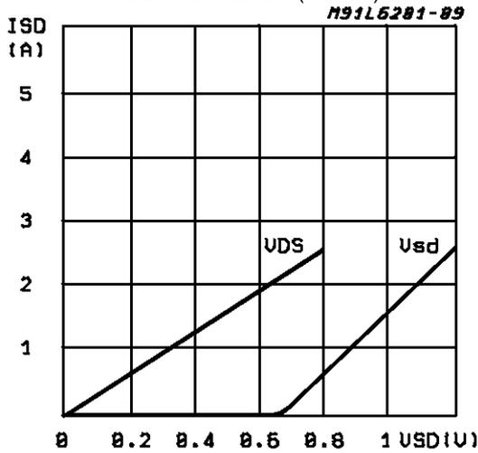
Figure 6b: Typical Diode Behaviour in Synchronous Rectification (L6201PS/02/03)
