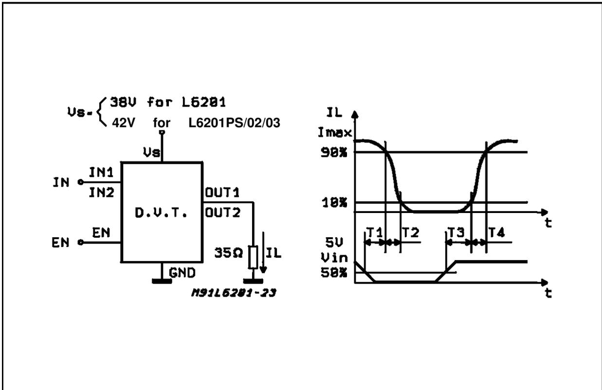
Figure 13: Sink Current Delay Times vs. Input Chopper
