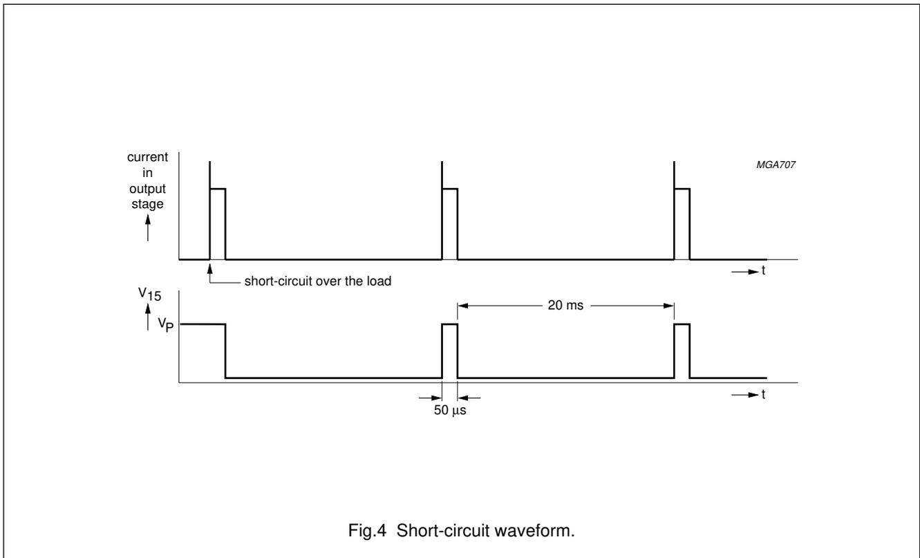
Fig.4 Short-circuit waveform.
