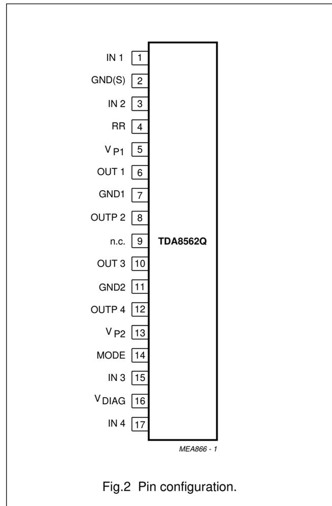
Fig.2 Pin configuration.
