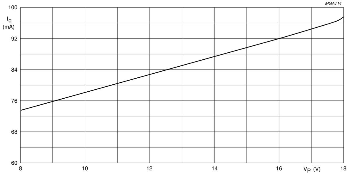
Fig.13 Quiescent current as a function of supply voltage; R<sub>L</sub> = ∞.
