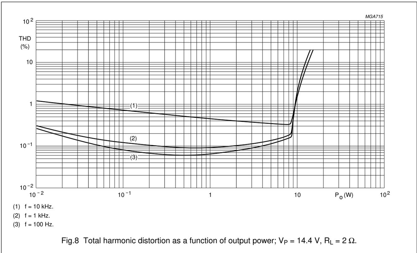
4 x 12 W single-ended car radio power amplifier with dynamic distortion detector and diagnostic interface
