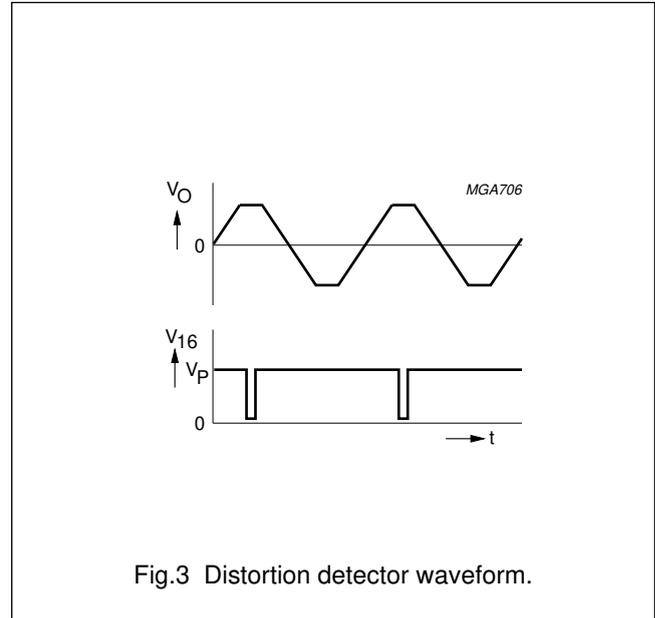
Fig.3 Distortion detector waveform.
