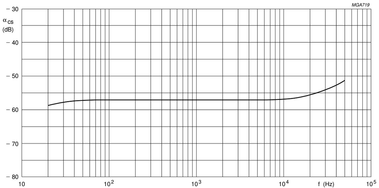
Fig.14 Channel separation as a function of frequency.
