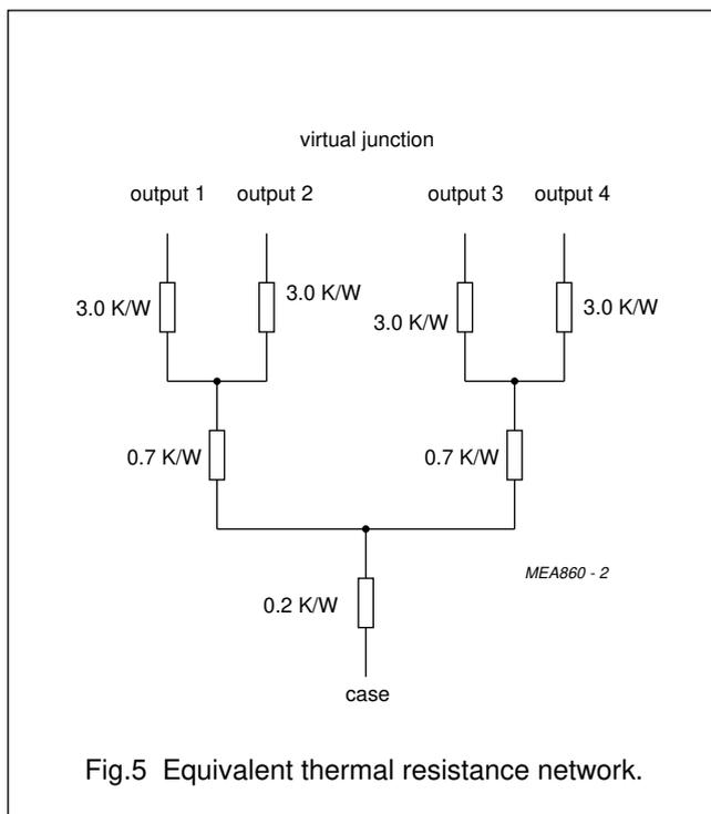
Fig.5 Equivalent thermal resistance network.
