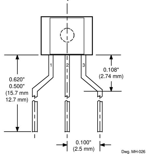
NOTE: Lead-form dimensions are the nominals produced on the forming equipment. No dimensional tolerance is implied or guaranteed for bulk packaging (500 pieces per bag).
