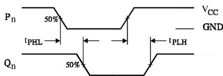
Figure 3. Switching Waveforms
