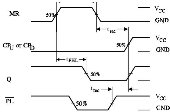
Figure 5. Switching Waveforms
