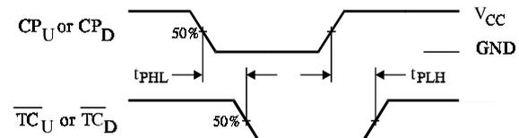
Figure 2. Switching Waveforms
