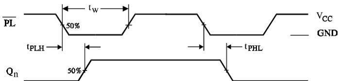
Figure 4. Switching Waveforms
