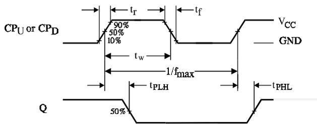
Figure 1. Switching Waveforms
