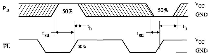
Figure 7. Switching Waveforms
