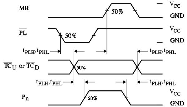
Figure 6. Switching Waveforms
