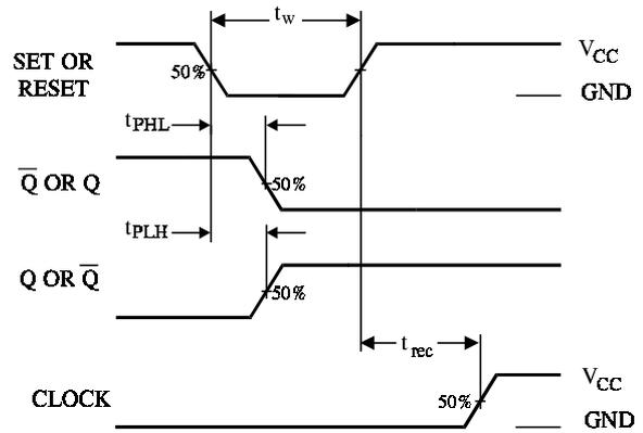
Figure 2. Switching Waveform
