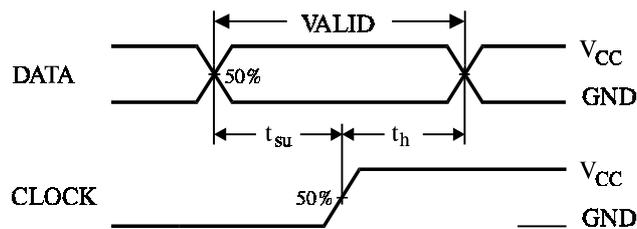
Figure 3. Switching Waveform
