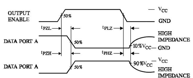
Figure 5. Switching Waveforms
