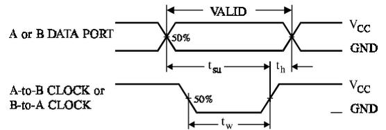
Figure 7. Switching Waveforms
