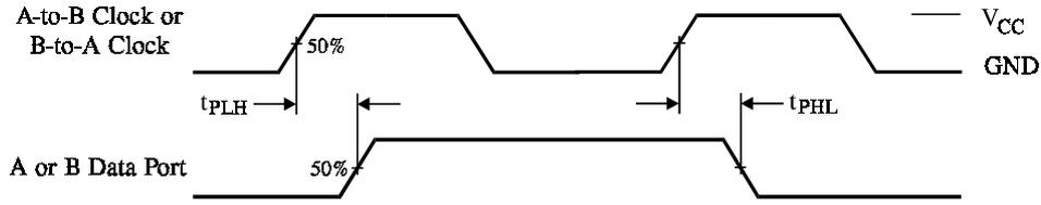
Figure 1. Switching Waveforms
