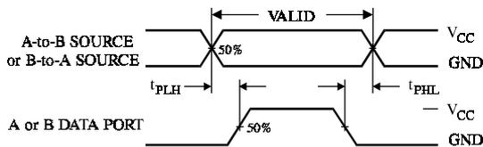
Figure 4. Switching Waveforms
