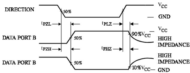
Figure 6. Switching Waveforms
