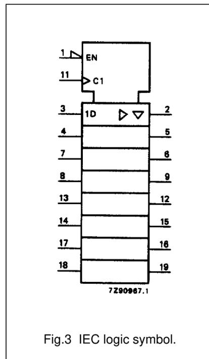
Octal D-type flip-flop; positive edge-trigger;
