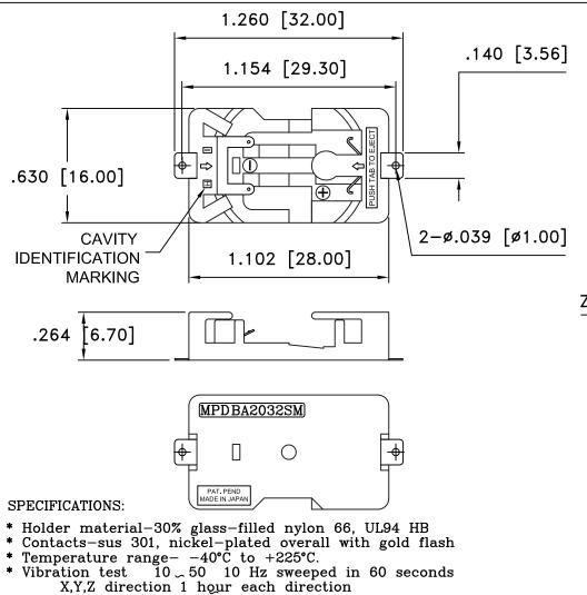
AUTH DR. CK. SYM REVISION RECORD Date ADDED "ROHS COMPLIANT" 11/05/05 ADDED PATENT NUMBER T.B. B.S. 2/11/06 2/17/07 DIMENSION .140 WAS .138 T.B. B.S. B.S. 4/26/08 ADDED SOLDERING SPEC. T.B. 6/27/08 MATERIAL WAS UL94V-0 T.B. B.S. 4/02/10 ADDED MARKINGS
