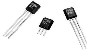
2SS52M Series position sensors have a built-in magneto-resistive bridge integrated on silicon and encapsulated in a plastic package. The integrated circuit also includes a band-gap regulator and a digital output that will respond to very low magnetic fields. Though the signal is identical to our digital Hall effect sensors, it can be achieved by magneto-resistive sensors at much greater sensor-to-magnet distances.
