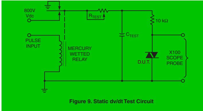
1. The mercury wetted relay provides a high speed repeated pulse to the D.U.T.
